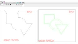
Mould produced using CAD/CAM. Students draw mould shape on 2D Design and this is laser cut ready for casting.
