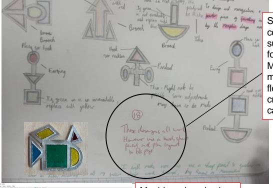
Students must consider the suitability of design for manufacture. Molten pewter must be able to flow within the void created by the diecasting mould.
